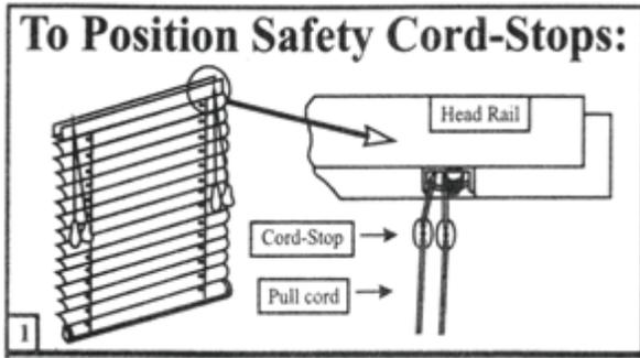
1. Install Blind as directed above, making sure head rail is securely fastened. Lower blind to maximum desired length and lock into place
