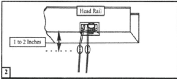
2. Measure the distance from head rail to cord-stops. If cord-stops are 1 to 2 inches below the head rail, no further adjustment is needed. Your wooden blinds are ready to use.
