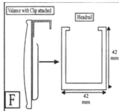
Hook valance clip with valance attached onto the top of the headrail.
