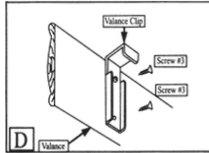
Screw valance clips onto back side of the valance with screws provided (screw #3)
