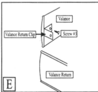
For Outside Mount: Screw one end of the valance return clip onto the valance using screw #3. Align the edge of the valance return with the valance. Screw the other end of the valance return clip onto the valance return.
