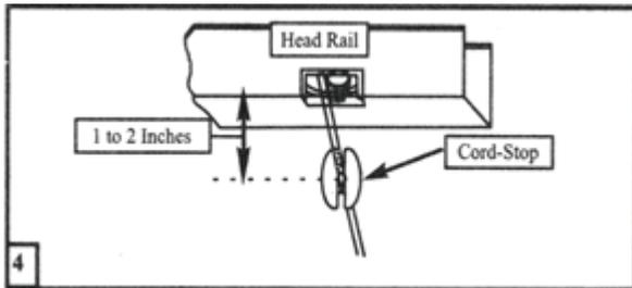
4. Push both the cord-stop and the loosen end knot toward the head rail until the cord-stop is 1 to 2 inches below the head rail. Hold cord-stop in place and pull firmly on pull cord to re-tighten knot. Repeat steps 2, 3 & 4 for each cord-stop.
