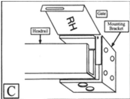
Push rail into brackets. Then press gate to close brackets.
